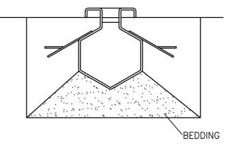
Backfill pocket until backfill is at finished floor level less the floor finish thickness to be applied.
